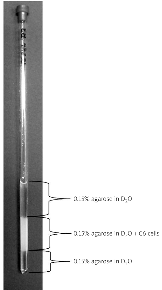
Fig. 1. Photograph of cells and agarose inserting 3-layers scheme inside the NMR tube.
